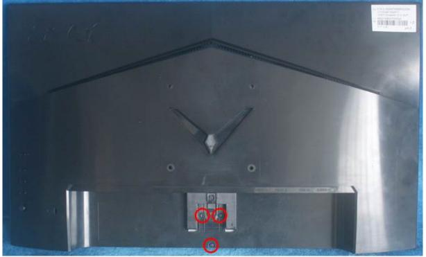
S2. Remove the rear cover. Use a tool to open all latches. (Be careful the position of the key board.)
