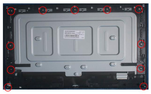
S4. Put the mainframe on the panel, connect cables (mainboard to panel and the power board to panel). Assemble the speaker. And paste all tapes.
