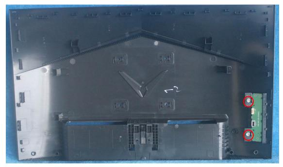
S6. Connect the pin (LED board / Key board), the pin (Key board to mainboard) .Use the screws to lock the rear cover.
